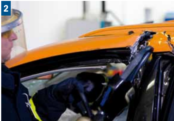
Cutting the B and C pillars
