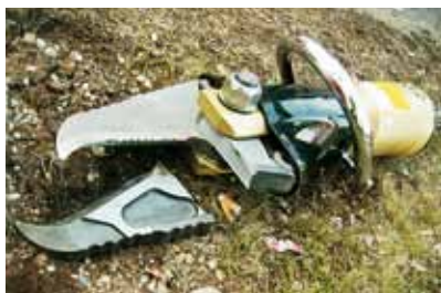
Reinforced A pillar (top) leaves a cutter in pieces
