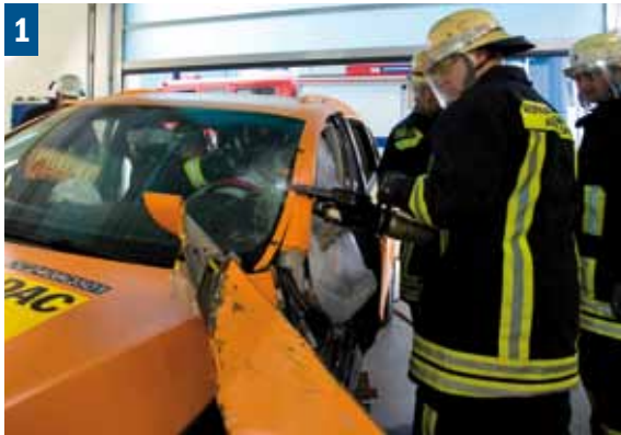
Removing the driver's door and cutting through the A pillar
